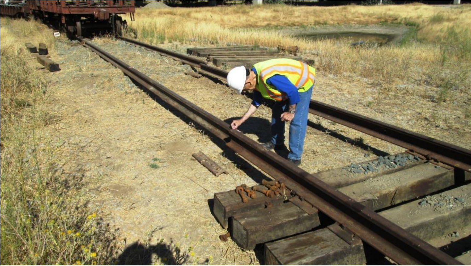
"On your marks!" Harry G. marks measuring points on the rails
