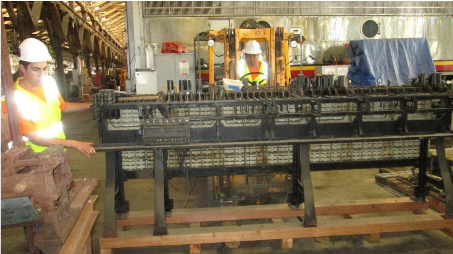
Weston and Anthony find a new home for the interlocking mechanism being restored by Team Signals
