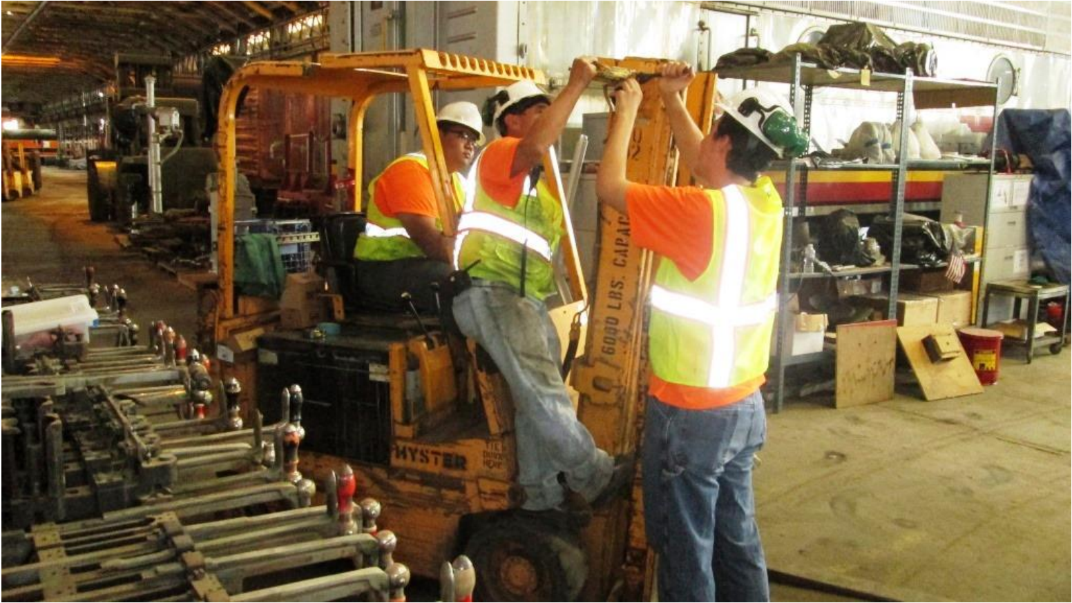
Joe and Weston install the new LED work-lights on the Hyster forklift
